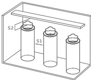
**Figure 5** Capacitor installation drawing
