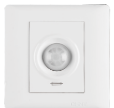
100W 1- Gang Infrared Snesor Time-delay Switch(Two-wire system. Control Filament Lamp. Energy Saving Lamp)
