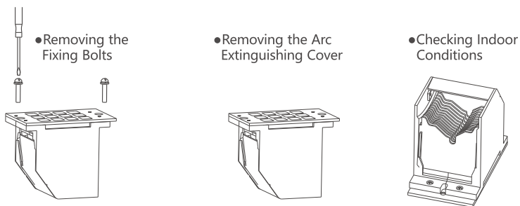
Fig59 Inspection for Arc Extinguishing Chamber
